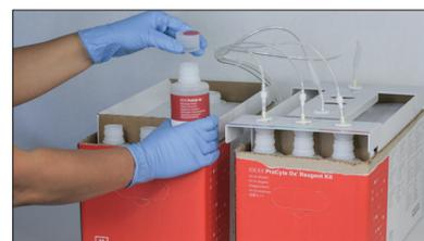
5. Place the quick-connect top onto the reagent kit, ensuring the probes are inserted into the 3 reagent bottles, the system diluent, and the waste container.
