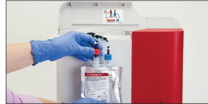
4. Place the stain pack upright into the compartment, ensuring the cords are in front of the stain pack inside of the compartment and that the stain packs are not crumpled. Then close the cover.
