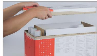
4. Remove the caps from the 3 bottles, system diluent, and waste container (use the cap remover in the original accessory kit, if necessary) and set them aside. Verify the order of the bottles is correct by matching the colour on the bottle labels with the colours on the shelf.
