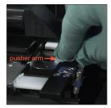
Using a new rinsed alcohol prep pad, clean the left side of the pusher arm 5 times (ensuring the right edge of the track is cleaned thoroughly), and then dry it with a new dry optical tissue.
