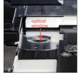
6b. Using a new alcohol prep pad (not rinsed), clean the optical window using a circular motion (3–4 times) and then dry it in a circular motion with a new dry optical tissue.
