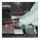
6a. Using a new rinsed alcohol prep pad, clean the optical stage and track repeatedly to remove all debris. Then dry with a new dry optical tissue.
