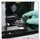
9. Return the waste bin, centrifuge shield, and cartridge holder to their locations in the Analyser.
