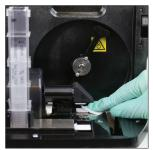
8. Using a new alcohol prep pad, clean the move arm and then dry it with a new dry optical tissue.
