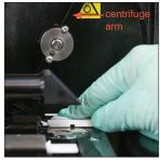
Gently move the centrifuge arm to the left and inspect the area below it for debris. If it's dirty, use a new alcohol prep pad to clean it and then dry it with a new optical tissue.
