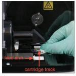
Using a new alcohol prep pad, clean the cartridge track and the white feed arm thoroughly. Then dry them with a new dry optical tissue.
