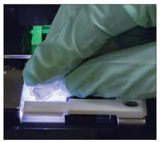
Open the Analyser door. Then, with gloved hands, use an optical tissue to absorb urine on top of the cartridge.
