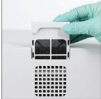
10. Remove the fan filter on the back of the Analyser, rinse it thoroughly with warm water, pat it dry with a paper towel, and return it to its location in the Analyser.
