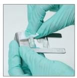
Remove the cartridge holder, clean it with a new alcohol prep pad, dry it with a new dry optical tissue, and then set it aside.
