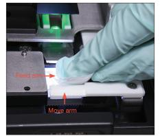
3. Using a new alcohol prep pad, clean the feed arm (dispense area), including the front of the move arm. Then dry the components with an optical tissue.
