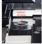
6b. Using a new alcohol prep pad (not rinsed), clean the optical window using a circular motion (3–4 times) and then dry it in a circular motion with a new dry optical tissue.
