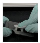
Remove the cartridge holder, clean it with a new alcohol prep pad, dry it with a new dry optical tissue and then set it aside.
