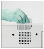
10. Remove the fan filter, rinse it thoroughly with warm water, pat it dry with a paper towel and return it to its location in the analyser. Then on the SediVue Dx Cleaning Guide screen, tap **Done** to power on the SediVue Dx.
