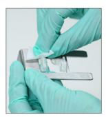
Remove the cartridge holder, clean it with a new alcohol prep pad, dry it with a new dry optical tissue and then set it aside.
