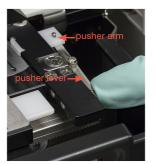
5. Press the pusher lever to the left and repeat step 4 on the right side of the pusher arm using a new rinsed alcohol prep pad.
