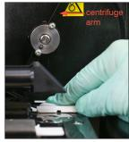
Gently move the centrifuge arm to the left and inspect the area below it for debris. If it's dirty, use a new alcohol prep pad to clean it and then dry it with a new optical tissue.
