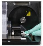
Using a new alcohol prep pad, clean the move arm and then dry it with a new dry optical tissue.
