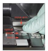
6a. Using a new rinsed alcohol prep pad, clean the optical stage and track repeatedly to remove all debris. Then dry with a new dry optical tissue.
