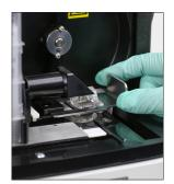
Return the waste bin, centrifuge shield and cartridge holder to their locations in the analyser.
